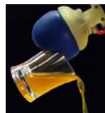
Jamming Gripper Cicigo Univ.+iRobot
